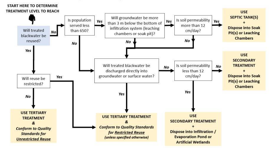
Figure 2: Treatment level to reach for any effluent containing blackwater flowchart
